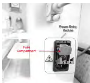
Figure 64: Power Entry Component with Fuse Compartment
