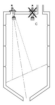
D - On fluid-like solids, aim transducer perpendicular to material surface.
