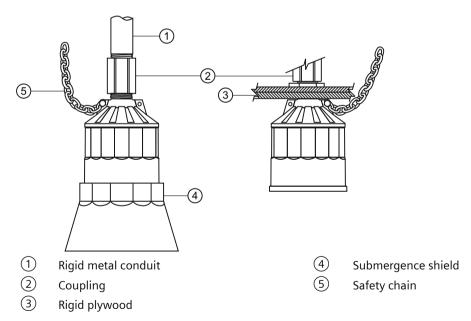
Transducer with submergence shield, used in applications where flooding is possible.
