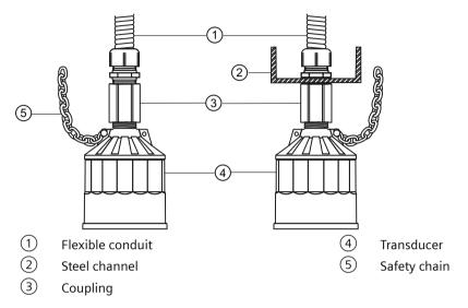
Flexible conduit mounted transducer should not be subjected to wind, vibration, or jarring.
