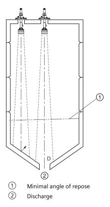
E - On dual discharge bins, aim each transducer at the discharge point.
