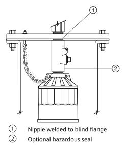
Flange, gasket, and hardware supplied by customer.
