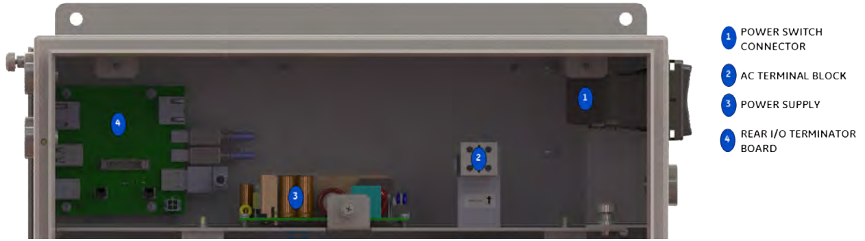
Figure 46: Electronics Enclosure (Top Shelf) — M9 and M9 e On-Line Analyzers
