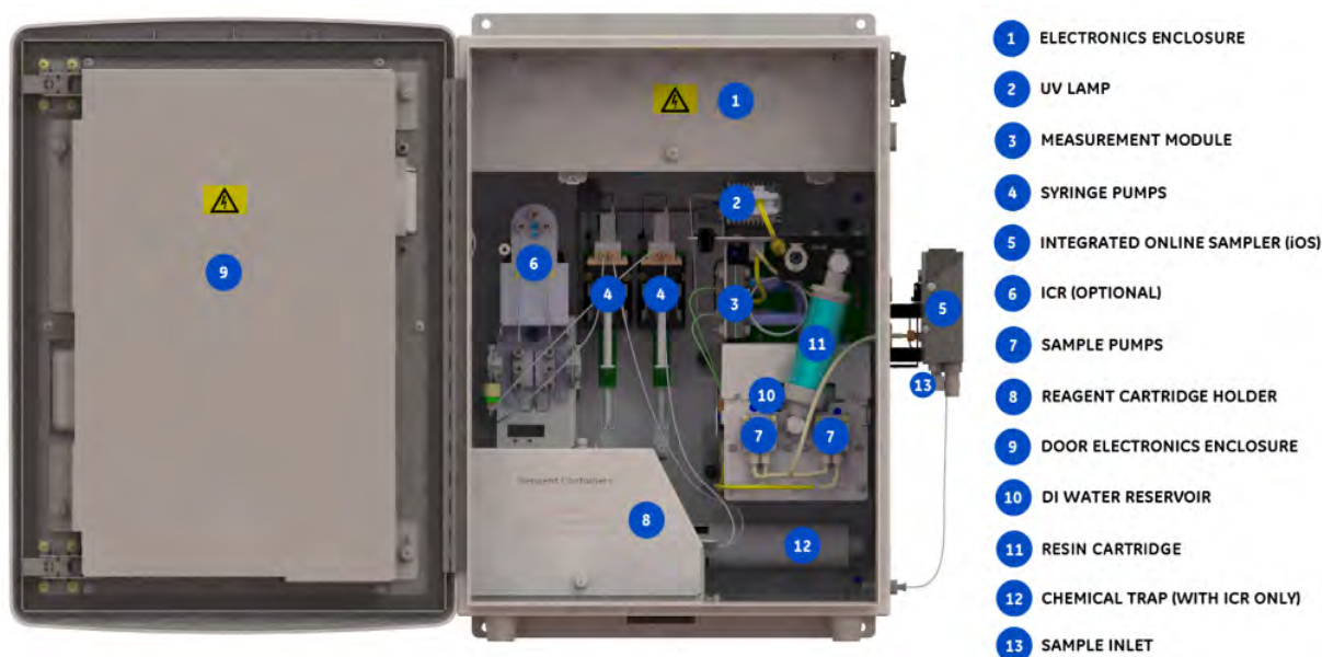
Figure 45: Interior Overview — Sievers M9 and M9 e On-Line TOC Analyzers
