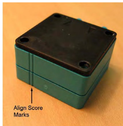
Figure 79: Aligning the Pump Plates
