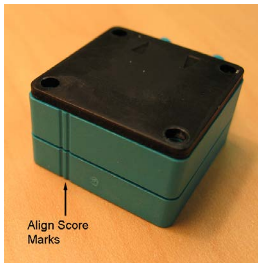
Figure 88: Aligning the Pump Head Plates
