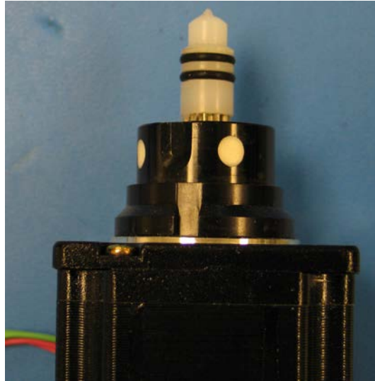
Figure 85: The High Pressure Valve Seal — Before Removal
