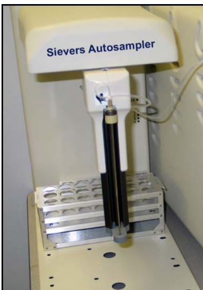
Figure 18: Lowering the Sievers Autosampler Arm
