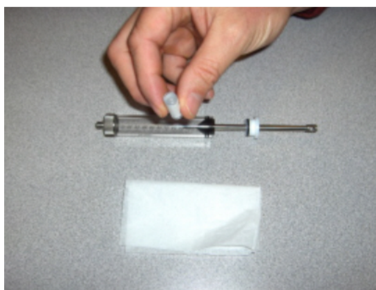
Figure 78: Removing the Stopper
