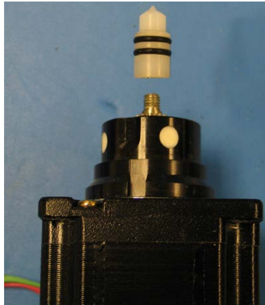
Figure 86: The High Pressure Valve Seal — After Removal
