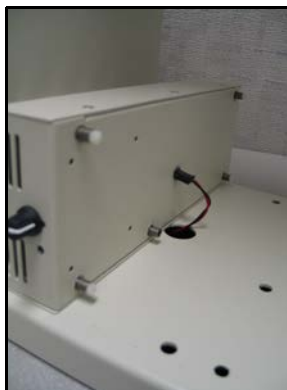
Figure 13: Connecting the Stirring Plate Wiring
