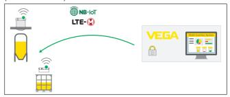
Fig. 14: Remote access from VEGA Inventory System via NB-IoT or LTE-M to the sensor
