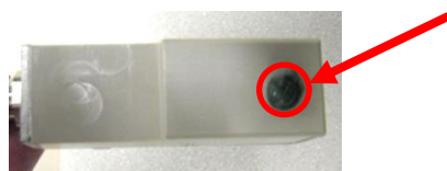
Figure 11: Transducer with an approx. peanut-sized drop of coupling gel
