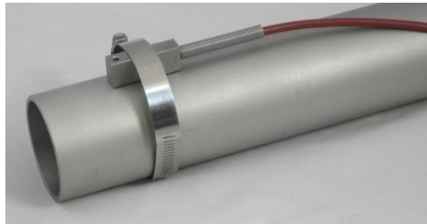
Figure 22: At pipe mounted Pt100
