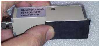
Figure 10: XUC-FW F10 with acoustic coupling pad
