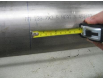
Figure 16: Mark the distance between transducer
