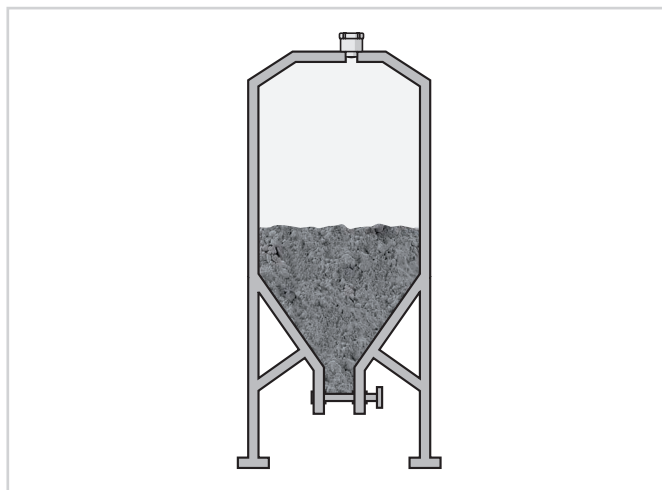
Level measurement in the building material silo
