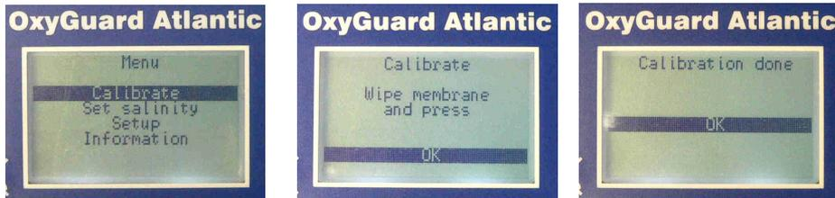
*For the best results make sure the probe has the same temperature as the air. Atlantic will remind you to wipe the probe*
