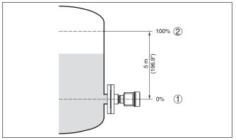
Fig. 29: Parameter adjustment example Min./max. adjustment, level measurement
