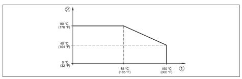
Fig. 38: Temperature derating VEGABAR 83, version up to +150 °C (+302 °F)
