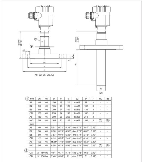
Fig. 50: VEGABAR 83, flange connection 180 °C/200 °C (METEC® measuring cell)
