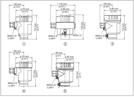
Fig. 43: Housing versions in protection rating IP66/IP67 and IP66/IP68 (0.2 bar), (with integrated display and adjustment module the housing is 9 mm/0.35 in or 18 mm/0.71 in higher)
