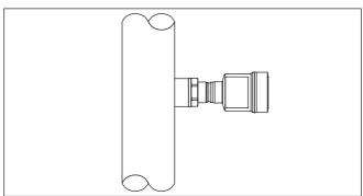
Fig. 2: Process pressure measurement VEGABAR 83
