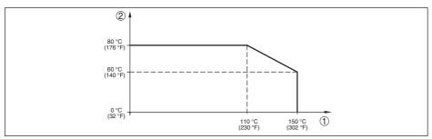
Fig. 39: Temperature derating VEGABAR 83, version up to +150 °C (+302 °F)
