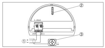
Fig. 18: Electronics and connection compartment - single chamber housing
