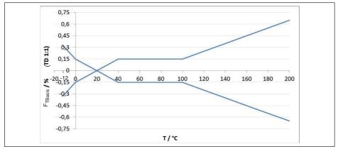
Fig. 35: Basic temperature error F<sub>TBasis</sub> at TD 1 : 1
