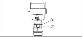
Fig. 9: Position of the filter element - Ex-d version
