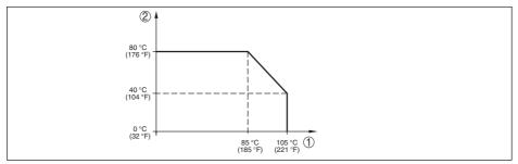
Fig. 37: Temperature derating VEGABAR 83, version up to +105 °C (+221 °F)
