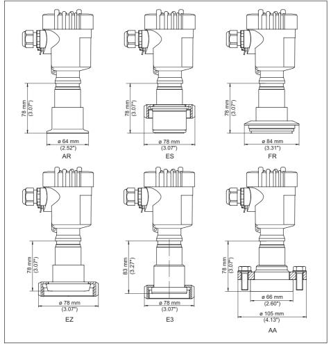
Fig. 48: VEGABAR 83, hygienic fitting 150 °C (METEC® measuring cell)
