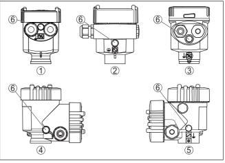
Fig. 8: Position of the filter element
