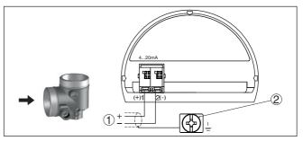
Fig. 20: Connection compartment - Ex-d-ia double chamber housing
