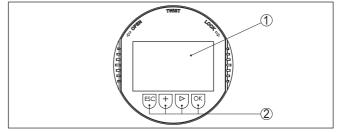
Fig. 27: Display and adjustment elements
