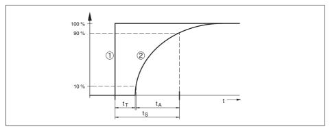
Fig. 33: Behaviour in case of sudden change of the process variable.  $t_{\tau}$  dead time;  $t_{A}$ : rise time;  $t_{S}$  jump response time
