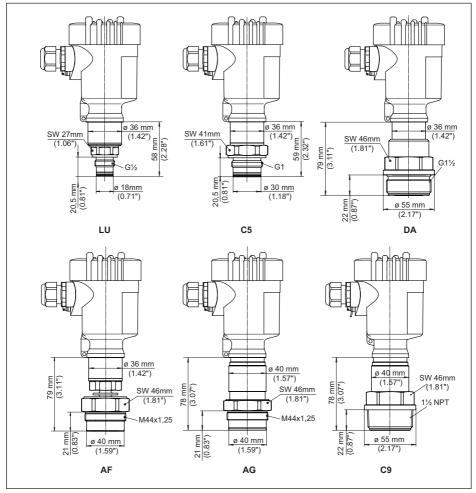
Fig. 46: VEGABAR 83, threaded fitting front-flush
