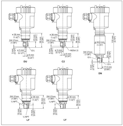
Fig. 45: VEGABAR 83, threaded fitting not front-flush
