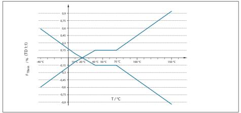
Fig. 34: Basic temperature error F<sub>TRasis</sub> at TD 1 : 1
