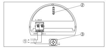
Fig. 25: Electronics and connection compartment - single chamber housing
