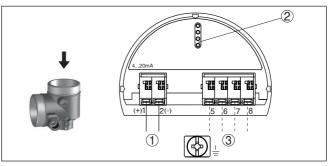
Fig. 19: Electronics compartment - Ex-d-ia double chamber housing
