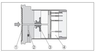
Fig. 6: Configuration of the METEC® measuring cell
