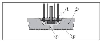
Fig. 4: Configuration of the measuring system with piezoresistive sensor element
