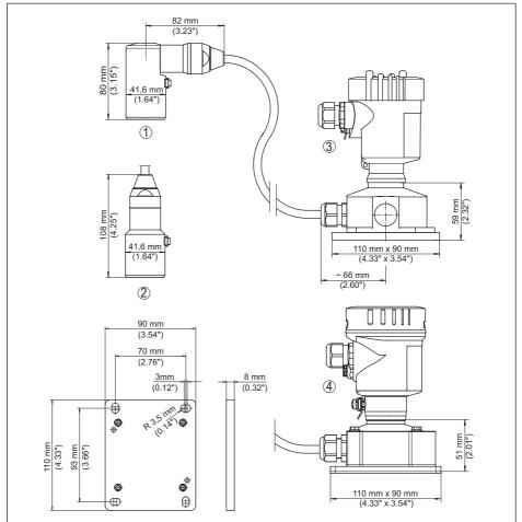
Fig. 44: VEGABAR 83, IP68 version with external housing
