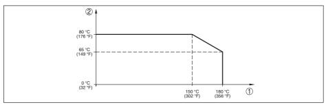
Fig. 40: Temperature derating VEGABAR 83, version up to +180 °C (+356 °F)
