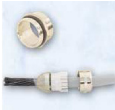
Figure 5b -Feed cable through dome nut and clamping insert -Fold braided shield over clamping insert -Make sure braided shield overlaps O-ring
